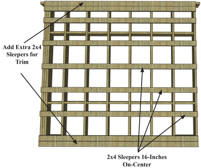
Add additional framing for railing posts, cut tiles, & extra sleepers for edge trim, where needed.
